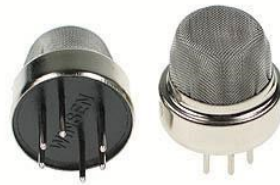
Fig -: Gas Sensor
