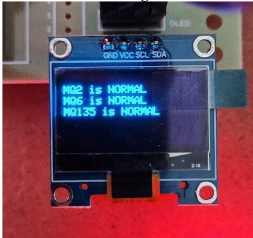
Fig OLED displaying normal state of gas sensors
