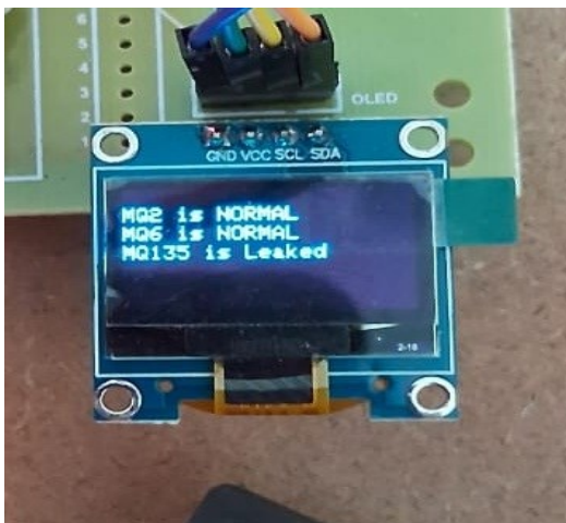
Fig OLED displaying leak status
